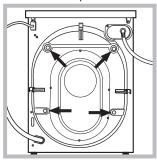
Remove the 4 protective screws (used during transportation) and the corresponding spacer, located on the rear part of the appliance (see figure).
